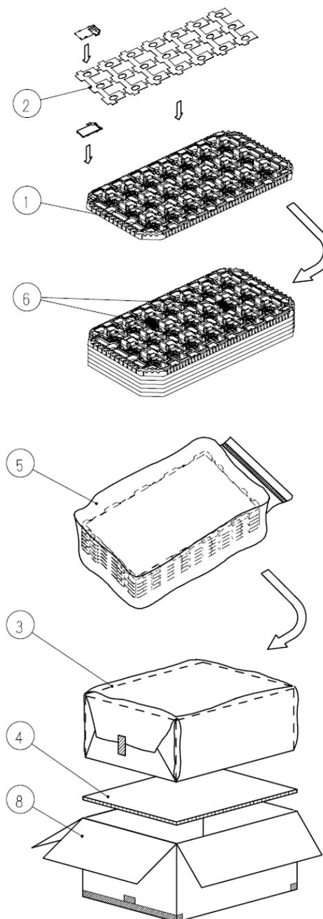
Step1. Each product is to be placed in one of the cut-outs of the tray with it's the LCD display side facing upward, and foam-sheet is put on products.(21 pieces/1 step)
