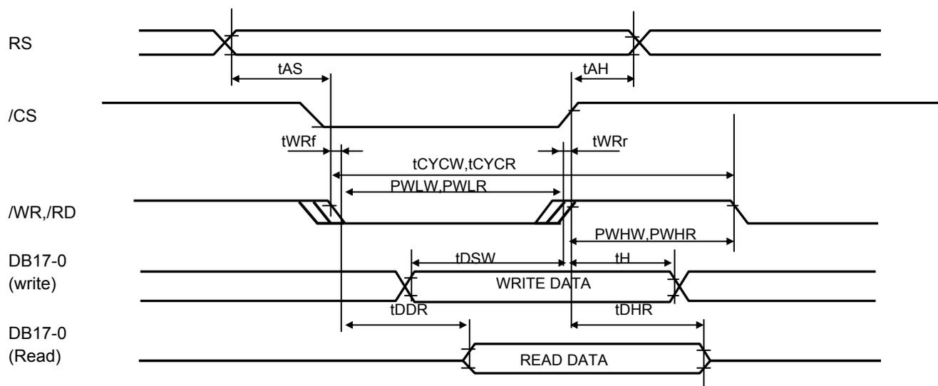
Note : PWLW and PWLR are determined by the overlap period of low /CS and low /WR or low /CS and low /RD.
